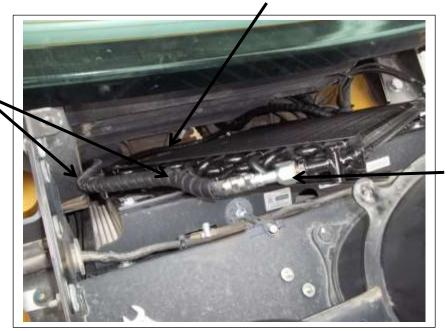
Slide the condenser and the 5/16" hose down the front of the oil cooler with the fitting side of the condenser tilted up as shown. Connect the 13/32" fitting ( with "O" ring) to the top fitting on the condenser. Tie wrap the 13/32" hose to the side of the condenser as shown. Slide the condenser fully back into place. Make sure the condenser hooks the bottom bracket. Bolt the top of the condenser to the upper bracket with the 1/4" hardware provided.
