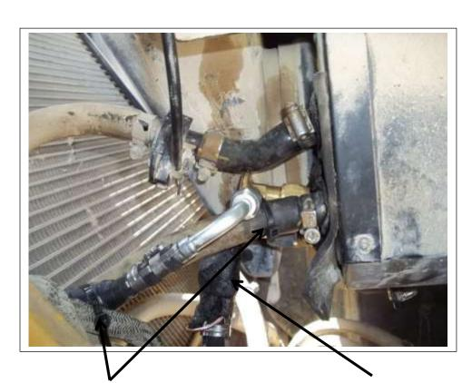
Secure all lines to prevent breakage from vibration
