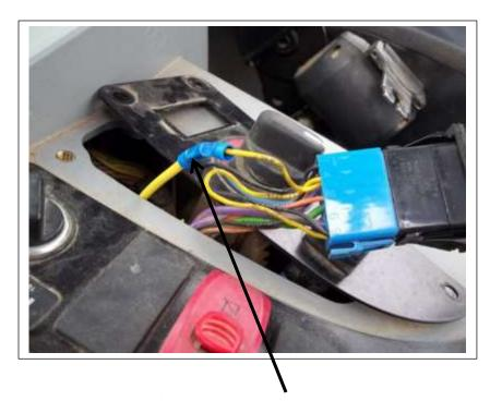
Butt connect the wire from the thermostat as shown, to the existing yellow wire # 521 that will be cut and stripped.
