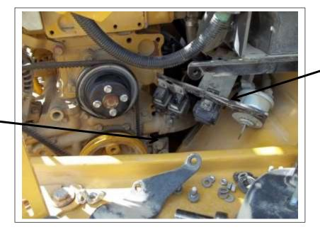
Unbolt this relay switch bracket to make enough room to slice the compressor down in front of the engine.
