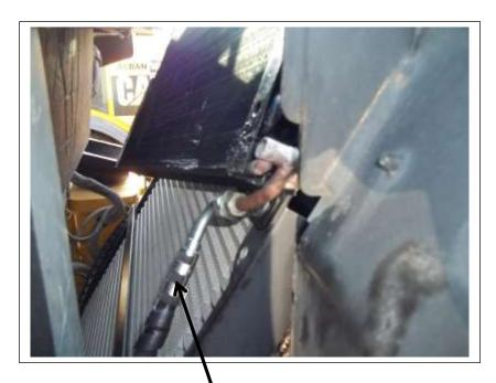
5/16" hose (64" long) mounted on the bottom fitting of the condenser going over to the drier on the right side of the radiator.
