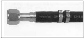
Step 5. Snap the cage into the groove on the nipple. The arms should extend over the hose length. When the cage has been correctly installed in the cage groove, the cage will be able to rotate in the groove. This step MUST be performed to ensure:
