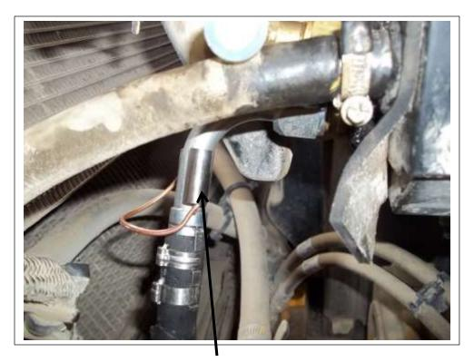
Expansion valve bulb clamp. Install as shown
