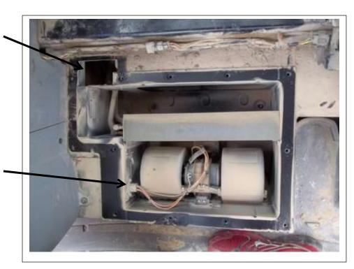
Lid removed. The blower box cannot be removed until the heater lines and blower wiring are disconnected. The access panel is on the side of the machine.
