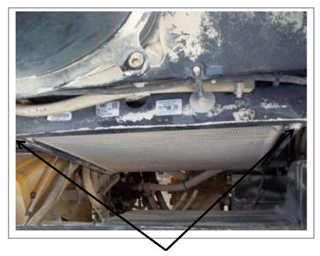
Remove these two bolts ( one on each side) at the top of the existing oil cooler.
