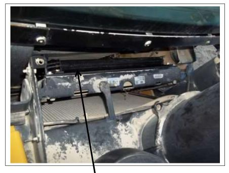
For cleaning, the top two 1/4" bolts can be removed and the coil pulled up. The hoses have been left long to allow for this cleaning procedure.
