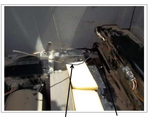
Set the heater box back into place in the cab. Be careful of the drain tubes when setting in place.
