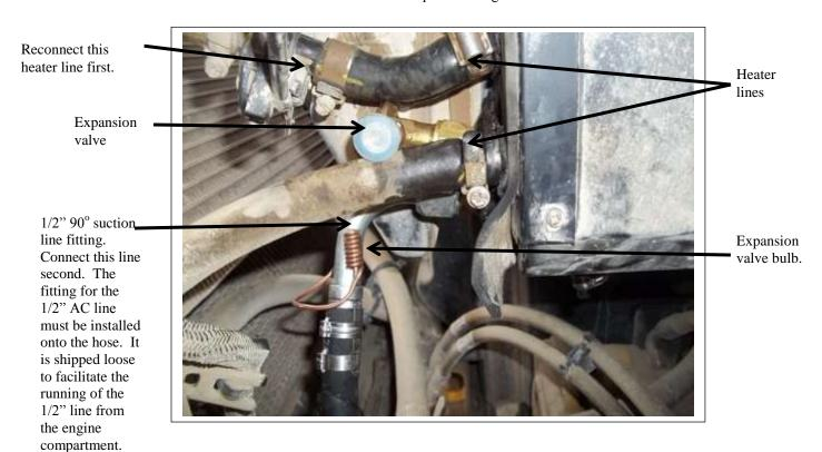
Reconnect the upper heater line with the heater control valve first. Connect the 1/2" AC line next for best access. Use stubby 1 1/6" and 7/8" wrenches to tighten. Don't forget the "O" ring. Reconnect the lower heater line.
