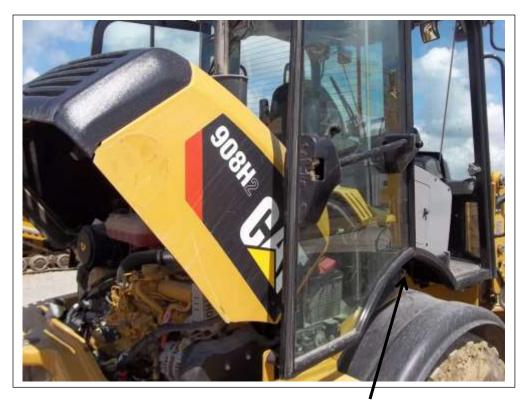
Remove this panel to get access to the heater hose connections. On the 906H2 machines, remove the plastic fender first.
