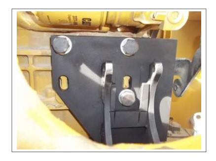
The compressor mount may appear a little different than shown however it will mount to the engine as shown. Hardware is provided in the kit.
