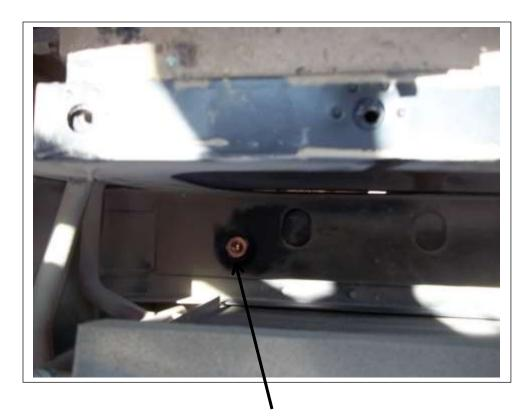
Drill out to 9/16" the two existing holes as shown and install the glue-in drain tubes into the bottom of the heater box. Use fast dry epoxy to glue in.
