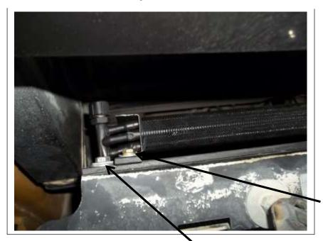
1/4" hardware bolting condenser to top bracket.
